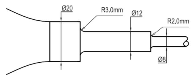
A round and rotating shaft made from AISI 1050CD is part of a powered machine. During application, a tensile load of force from 10N to 500N and a twisting force from 5.0Nm to 14.0 Nm are needed. If the machine is designed to for infinite life determine the safety factor for the proposed design. Use the Modified Goodman for fatigue analysis.
