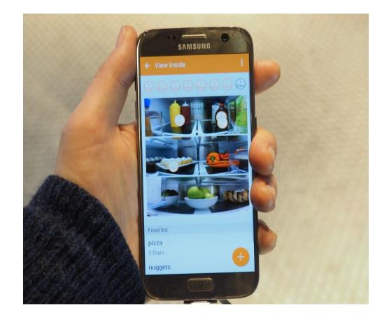
RFID readers in refrigerator can read the items inside and can stream the data to server and to the mobile devices. Server make analysis about the type of item and their expiry date, how stale the food will be in next one day, what's the condition of the food now, what all recipes can be prepared from the items in the fridge. User can get to see the items inside refrigerator using the camera inside the Samsung Hub.
