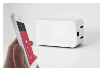
the Zuli Smartphone App. If 3 or more SmartPlugs are employed in the house, they can work together and determine the exact location of the user in the apartment. The App is the end-user interface, and allows to perform all the functionalities: monitoring, control and scheduling of the appliances.
