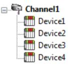
Each device appears under a single channel. In this configuration, the driver must move from one device to the next as quickly as possible to gather information at an effective rate. As more devices are added or more information is requested from a Device2 single device, the overall update rate begins to suffer.
