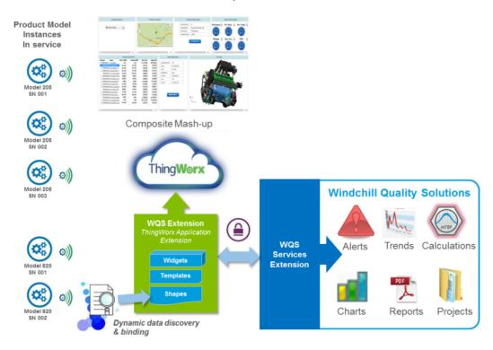
After you have imported the PTC Windchill Quality Solutions Extension into the ThingWorx Composer, a set of extensions is ready to use. These extensions allow you to use widgets to create mashups and applications that display data from PTC Windchill Quality Solutions.
