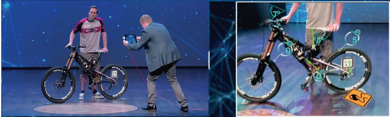
Figure 3 – Augmented Reality: Mountain Bike with Real-time Sensor Readings Superimposed (on iPad Screen at Right)
